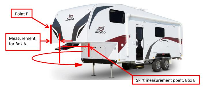
Place the end of a tape measure at the centre of the king pin (or centre of coupling for a Gooseneck) and move the other end around in an arc from fully forward to fully sideward to fully rearward. The LARGEST forward dimension is the measurement required for box A. Be careful to take in to account any point that projects further and could contact the vehicle cab, see point P above. The SMALLEST rearward measurement from the king pin centreline to the front skirt is to be entered in to Box B.
